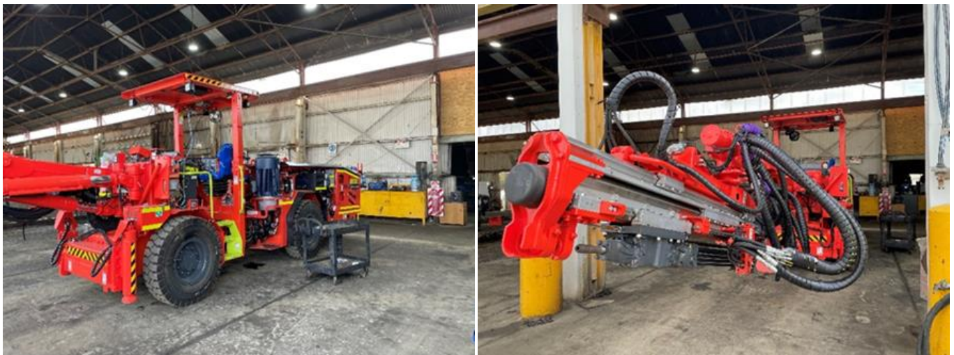
New, single boom jumbo being commissioned at Northern Operations
