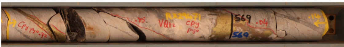
Figure 1: NQ core from diamond hole MFED095 with chalcopyrite - quartz veining in the sediment footwall adjacent to the Musket nickel deposit. This sample interval of 568.69 - 569.14 metres downhole returned 4.23% copper and 161.1 g/t silver.
