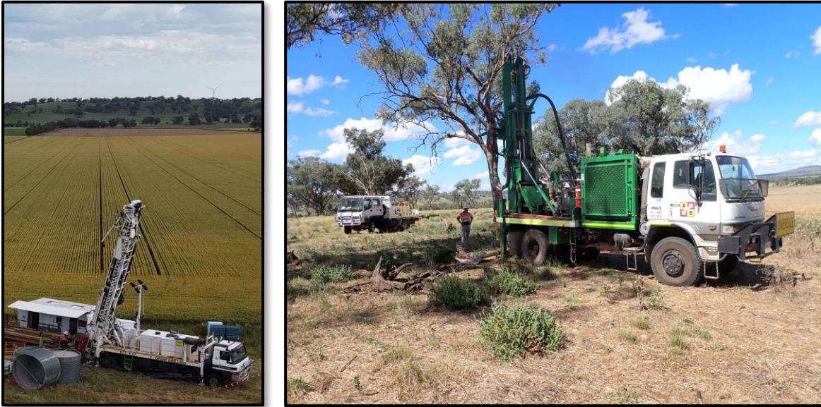
Figure 3: Diamond drill rig in December 2021 (LHS) and Aircore drill rig in January 2022 (RHS)
