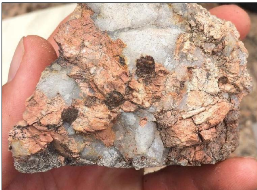
Figure 1. Garnet-bearing pegmatite float from tributary that contained 6.28 g/t Au & 0.83% TREO from stream sediment sampling (SRS13012).
