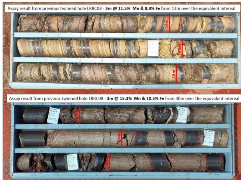
Figure 5. Recently drilled Black Canyon diamond core hole DDLR01 that is twinning historic RC hole LRR08 that intersected 37m @ 12.8% Mn and 10.5% Fe from 3m. Manganese bands are dark grey in colour. Note that the assays quoted are from the equivalent interval in historic drill hole LRR08 and assays for DDLR01 are pending. Error! Bookmark not defined.
