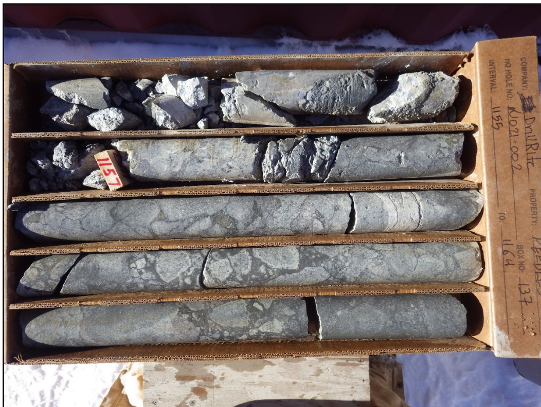
Figure 4. Brecciated unit in hole 21ND_002 showing altered andesite clasts within a pyrite-rich matrix (from 1,155ft to 1,164ft (352m to 354.8m))
