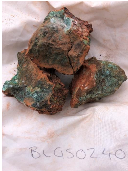
Figure 2: Outcropping mineralisation at the newly discovered Green Hills Prospect and rock chip sample BLG50240 which returned results of 24.30% Cu and 0.59 g/t Au.
