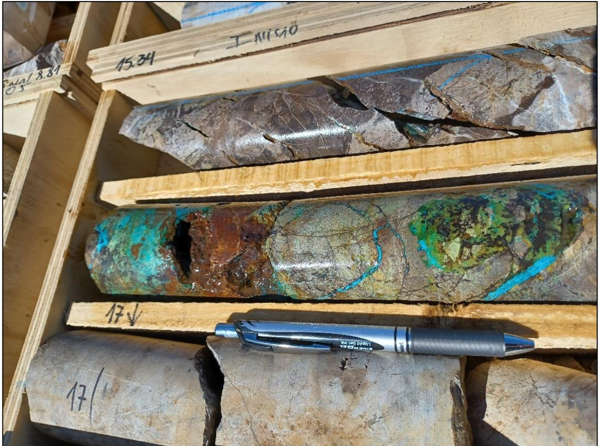
Figure 1: Visual copper mineralisation (malachite and chrysocolla) intersected in drillhole CMPDD006 at 16m downhole.
