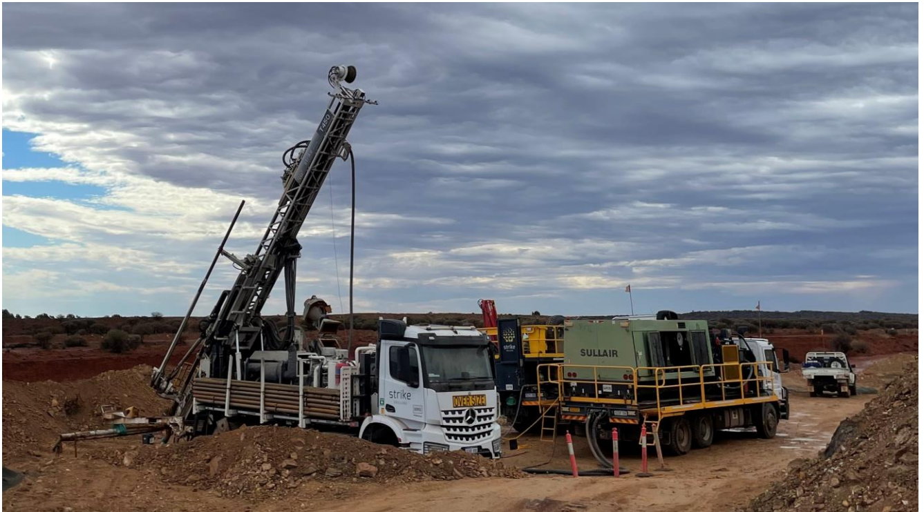
RC drilling by Strike Drilling at Cork Tree Well.
