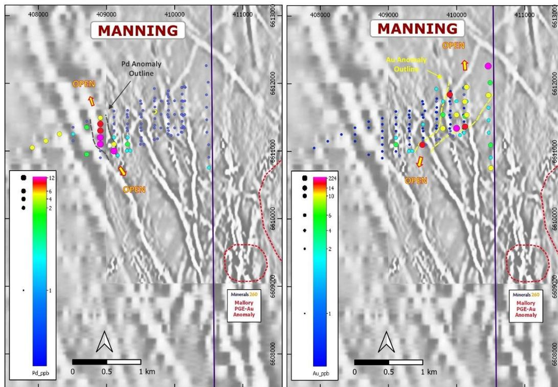
**Figure 5:** Manning Anomaly – 1<sup>st</sup> Vertical Derivative drone magnetic image with anomalous Pd (left) and Au (right) geochemical results
