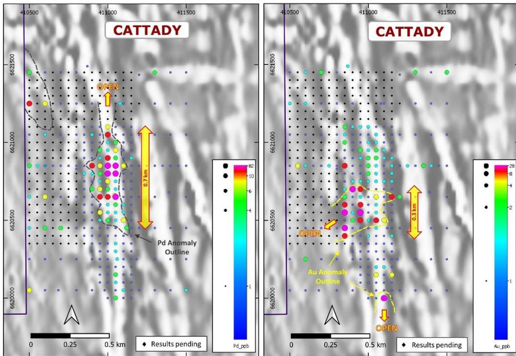
**Figure 3:** Cattady Anomaly – 1<sup>st</sup> Vertical Derivative drone magnetic image with anomalous Pd (left) and Au (right) geochemical results.
