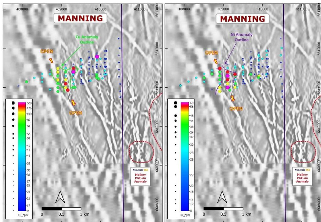
**Figure 6:** Manning Anomaly – 1<sup>st</sup> Vertical Derivative drone magnetic image with anomalous Cu (left) and Ni (right) geochemical results.
