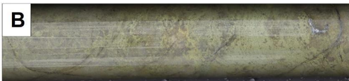
(B) Massive chalcopyrite >> pyrite with pyrite brecciation by later stage veinlets of coarse crystalline chalcopyrite. Minor quartz chalcopyrite infill lining of voids.
