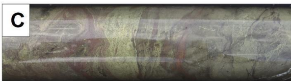
Figure 2: Revolver Drill hole 21DM DD003 6.95 m Massive Sulphide Body primary sulphide zone
