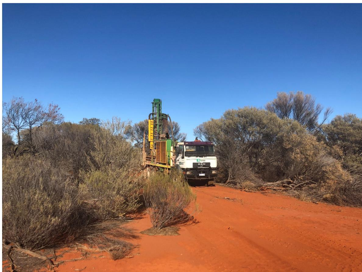
**Figure 2:** Aircore rig in action at Target 3 during the quarter
