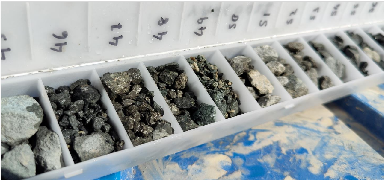
Figure 1. Drill chips from YARC0022 showing sulphide mineralisation.
