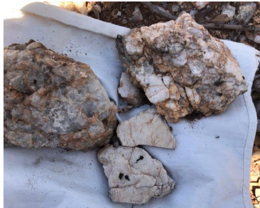
Figure 4 – Pegmatite sample from E45/5821, with possibly amblygonite as white secondary layer on quartz and feldspar (microcline) from southern part of tenure.
