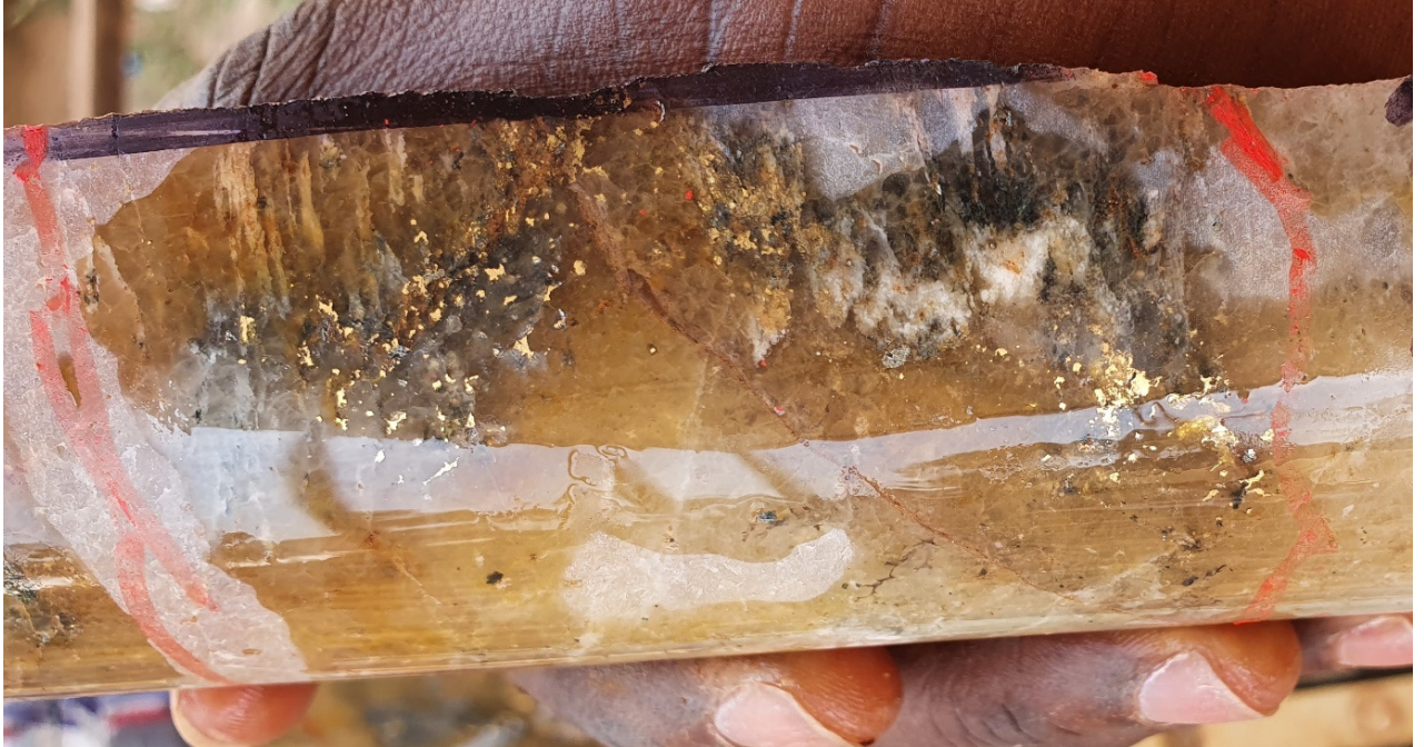
Figure 2: Diamond drill core of 1.1m at 2,853 g/t Au in ZDD895 on Section 14B
