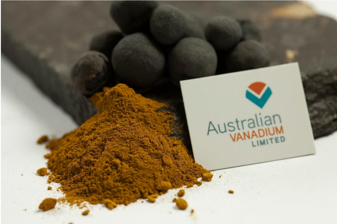
Figure 5 Sample of V_2O_5 precipitate generated from pilot program alongside roasted pellets and a vanadium ore sample.
