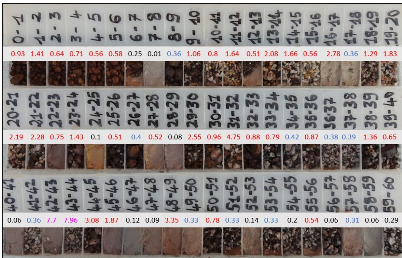
Figure 3: KRC047 drill chips from 0-60m showing gold grades (g/t). A new gold oxide intersection of 61m @ 1.2g/t gold was obtained from surface and will add ounces to the maiden Mineral Resource.
