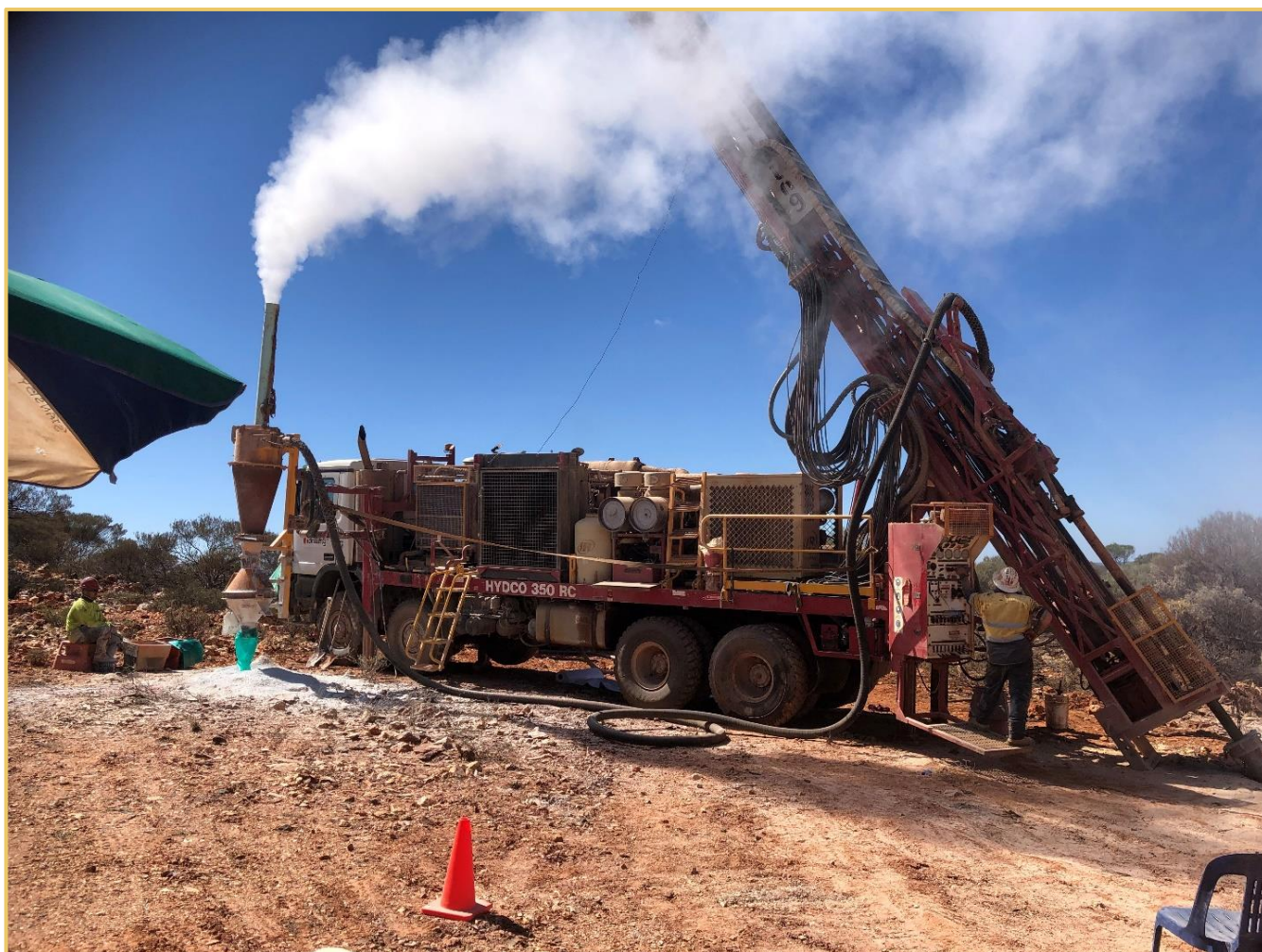
Figure 1 : RC Drilling Rig Drilling at Golden Crown.
