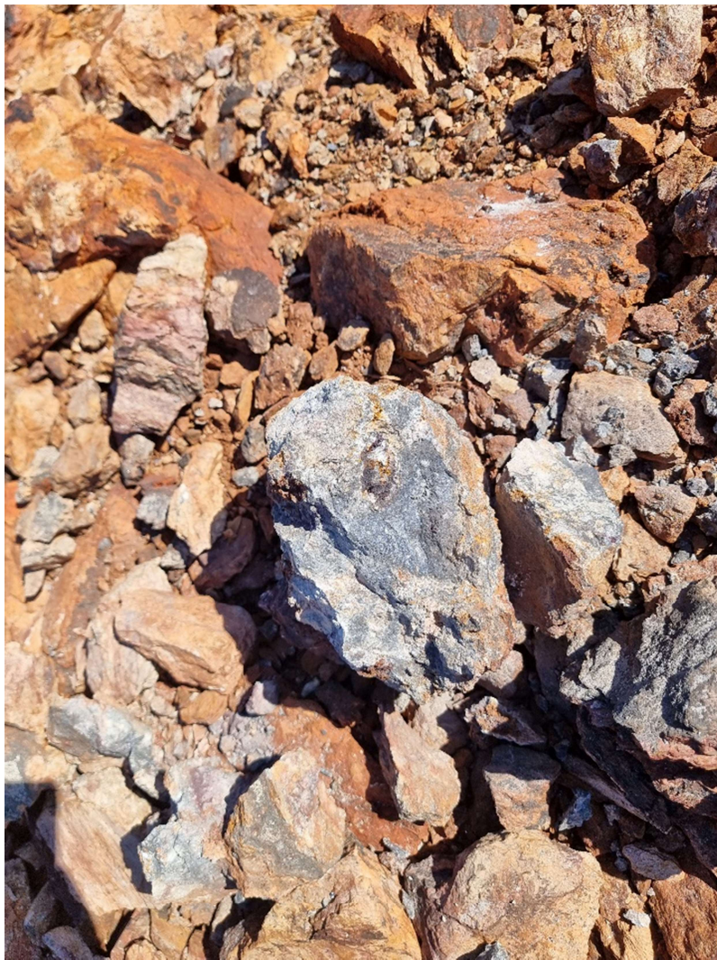
Figure 8: Highway Prospect showing high grade galena (grey colour) in chert and quartz. The rock in the center is about fist size.
