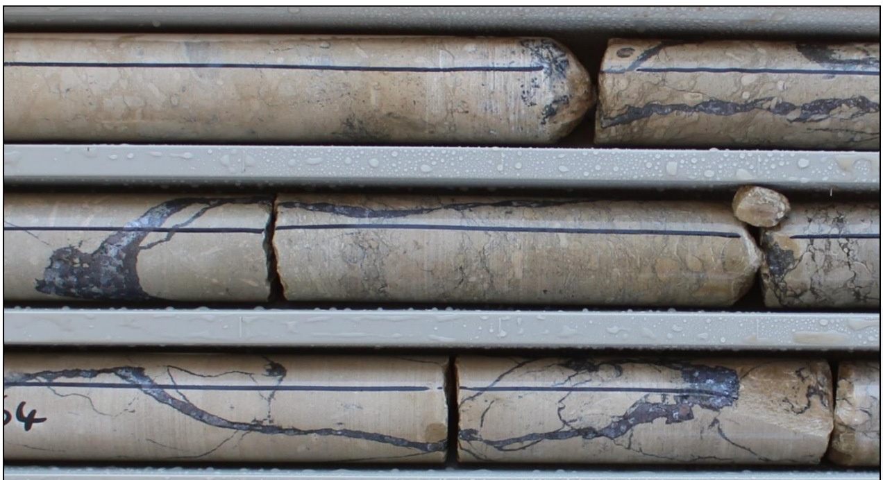
Figure 2: Sphalerite and galena-rich high angle-style mineralisation from hole EPDD2115: 1.00m @ 8.04% Zn + Pb from 38.00m.
