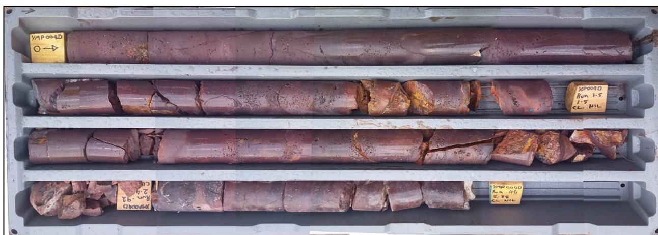
Figure 2. Hematite sandstone with hematite enrichment in drill hole YMP004D from surface to 2.88m depth.
