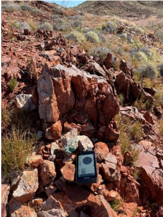
Figure 11: Outcropping mineralisation at the newly discovered Green Hills Prospect and rock chip sample BLGS0240 which returned results of 24.30% Cu and 0.59 g/t Au.
