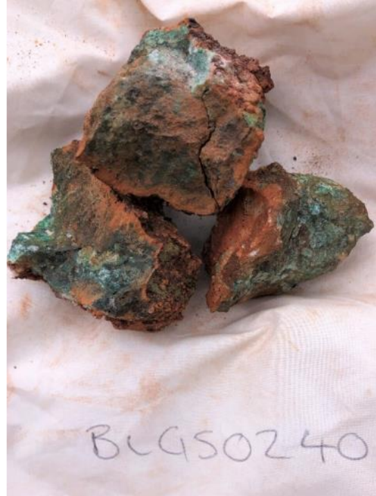
Figure 11: Outcropping mineralisation at the newly discovered Green Hills Prospect and rock chip sample BLGS0240 which returned results of 24.30% Cu and 0.59 g/t Au.
