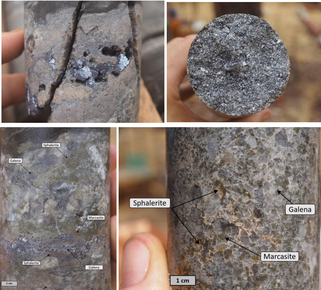
Figure 7 – Examples of mineralisation styles being encountered at Niamabimbou. Top Left: Coarse galena (lead sulphide) vein in NBDD018 within a dolostone at 34m; Top Right: Disseminated galena and sphalerite (zinc sulphide) in sandstone (8% galena + sphalerite logged) in NBDD006 at 24m; Bottom Left: Sphalerite (schalenblende style) and galena in NBDD016 at 23.5m; Bottom Right: Sphalerite, galena and marcasite in sandstone within NBD014 at 18m.
