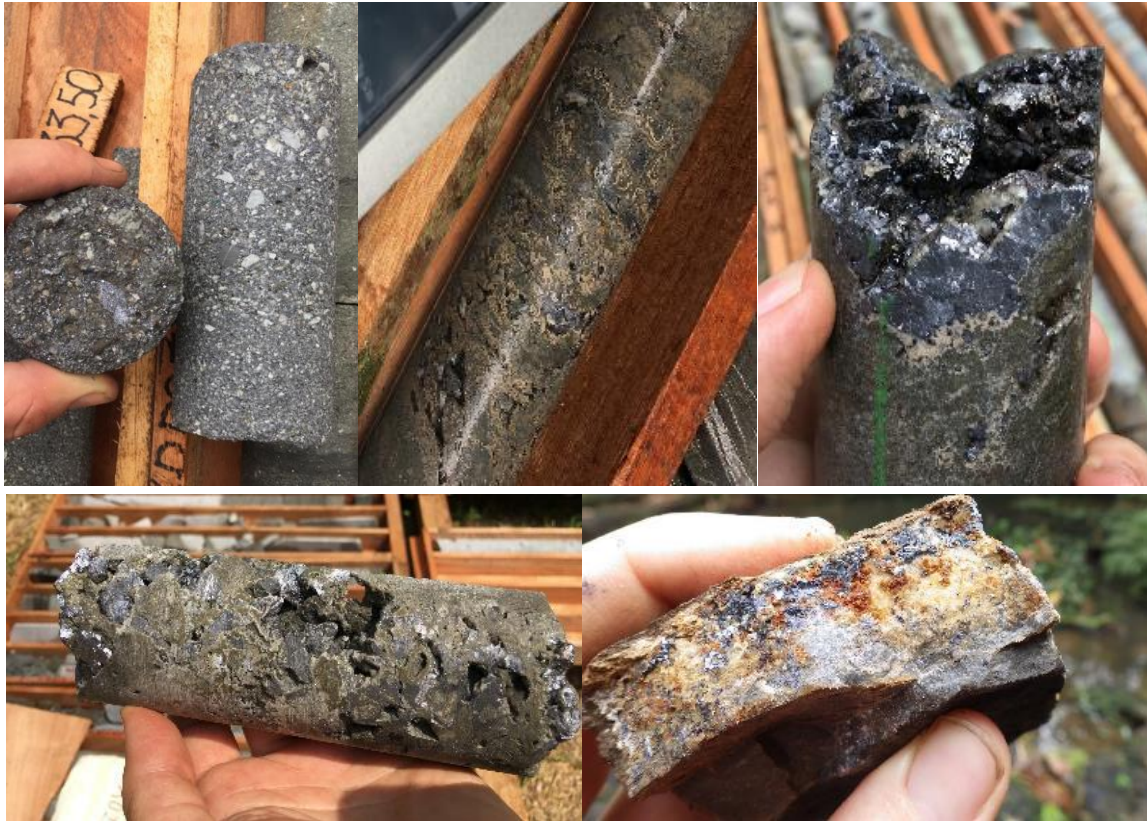
Figure 4: Sulphide mineralisation styles seen at Dikaki and surrounding area. Top Left: Disseminated coarse galena/sphalerite within sandstone/conglomerate unit (DKDD078); Top Middle: Concentric textured sphalerite and coarse galena within a breccia unit (DKDD001); Top Right: Galena and sphalerite within a breccia unit (BOD004); Bottom Left: Coarse textured galena, sphalerite and marcasite within the basal carbonate unit (DKDD013); Bottom Right: Outcrop of carbonate hosted galena and sphalerite.
