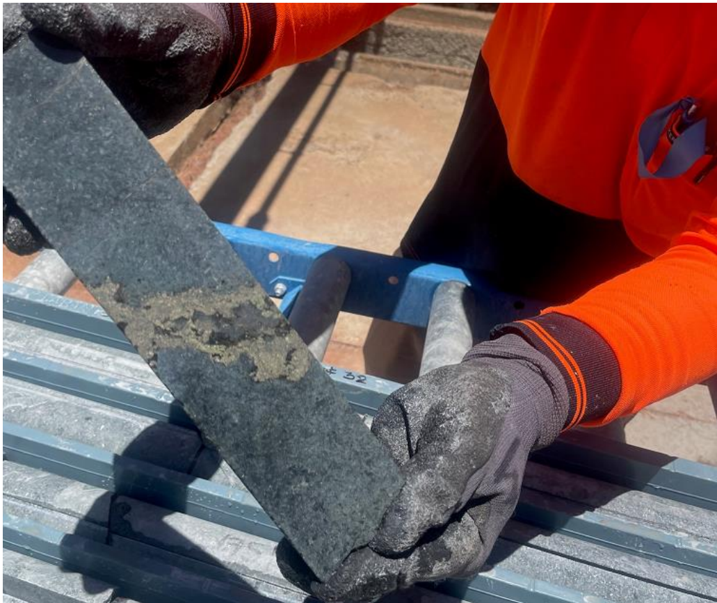
Figure 1: Mineralised core in the basal pyroxenite unit from CBDD063 at the Mossgiel Prospect
