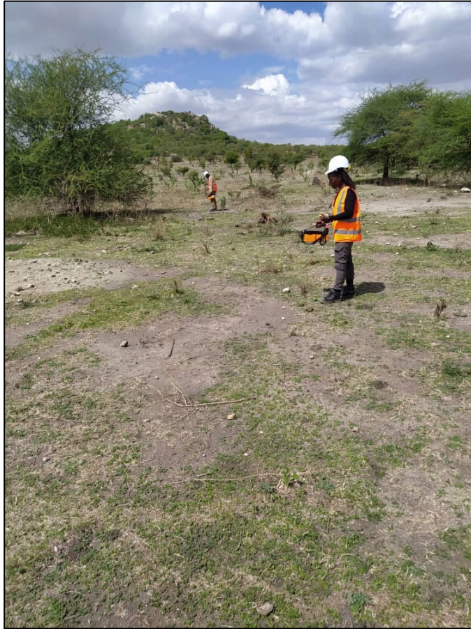
Figure 11: Gladiator resource exploration team conducting ground radiometric traverses south of Minjingu Hill
