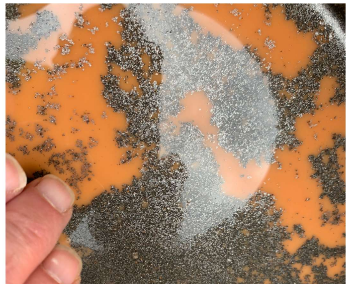
Figures 9 & 10: Very coarse-flake graphite in +600µm sample fraction (L), graphite floating on soaking drill sample (R)
