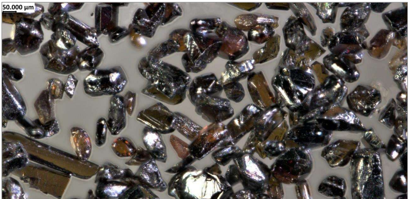
Figure 7: Photomicrograph of high purity rutile product 97.2% TiO 2
