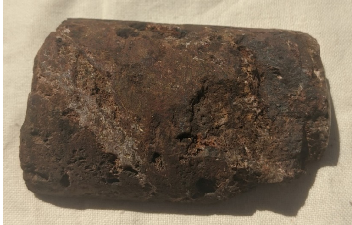
Figure 6: Gronnedal-Ika Sample (IVT 21 – 4) carbonatite, magnetite with 176 ppm Europium from 2.8m. (203.8 ppm Eu 2 O 3 )
