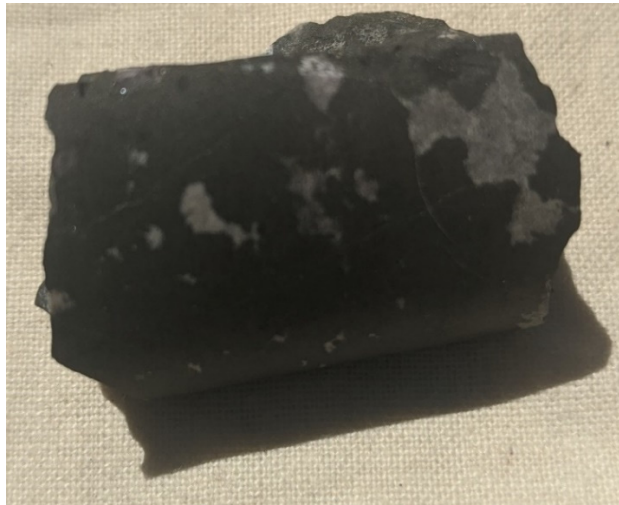
Figure 5: Gronnedal-Ika sample (IVT 21 – 1) magnetite from 71.73m with 3,670 ppm Niobium (5248 ppm Nb 2 O 5 )
