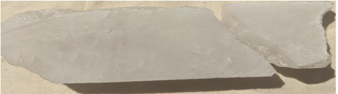
Figure 2: 99.7% SiO 2 in Sample IVT-21-5 of Quartz from 42.18m
