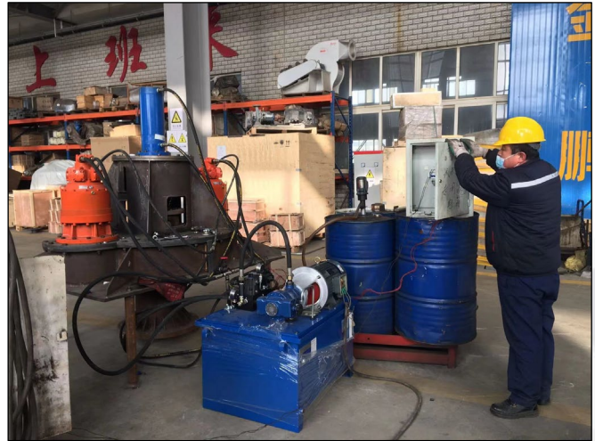
Figure 4: Vibration screen (left) and QA/QC testing of the thickener driver (right) before dispatching to Tanzania.
