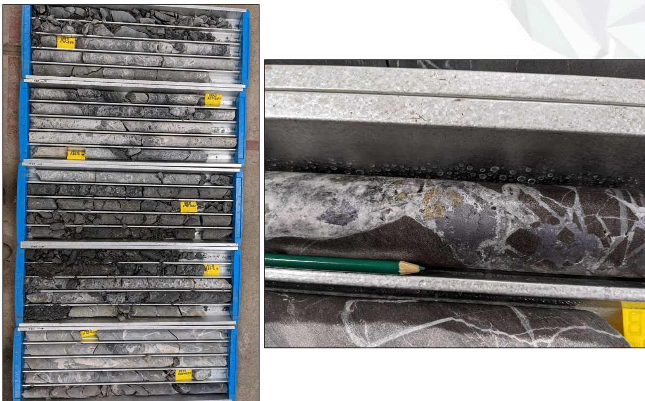
Figure 6: Left - Brecciated and altered "ore zone" in Drillhole BCRDD002 from 129m to 147m downhole. Right - galena (lead sulphide) and sphalerite (zinc sulphide) within the breccia zone.
