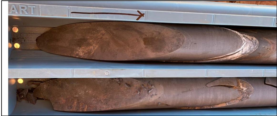
Image 10 | Native copper mineralisation 90.0m 21MDMT01
