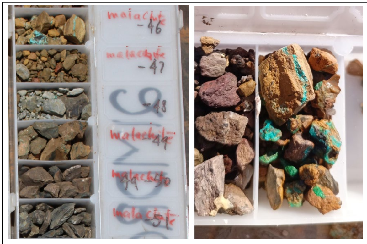
Image 4 | Malachite and Chrysocolla 46-51m 21MDRC016
