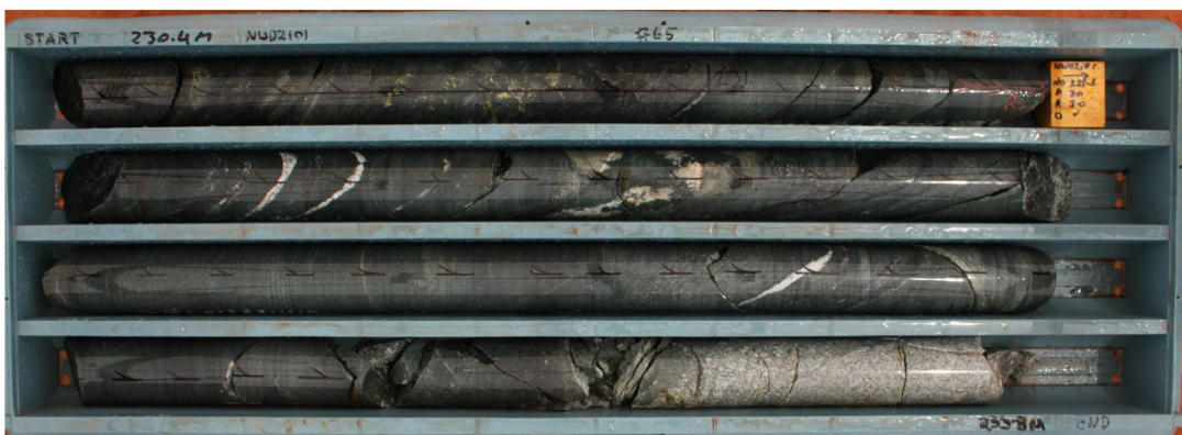
Image 14 | NWD2101: 229m to 231m; 2m @ 3.2% Cu, 0.6 g/t Au and 4.9 g/t Ag
