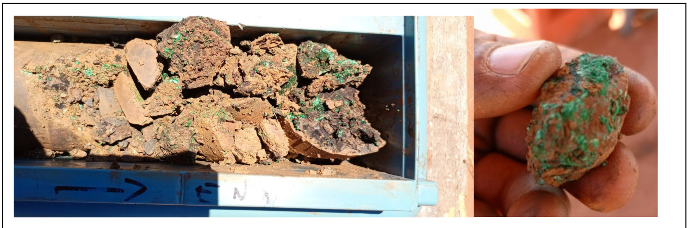
Image 9 | Malachite and chrysocolla mineralisation 87.2m 21MDMT01
