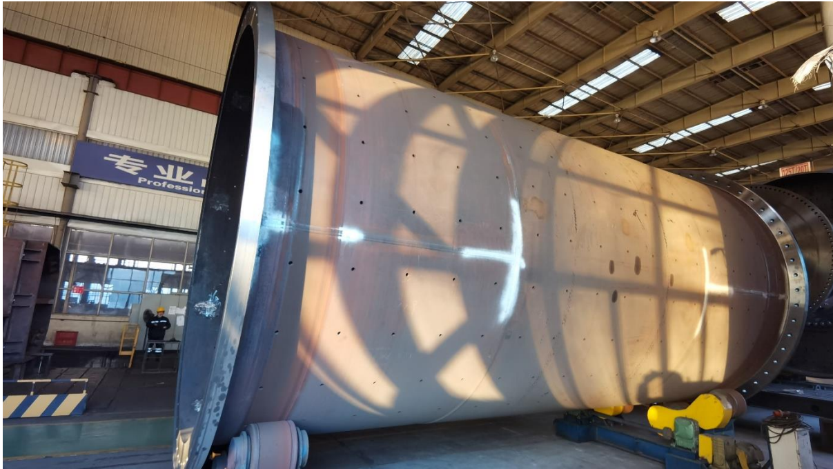
The Ball Mill Shell During Construction
