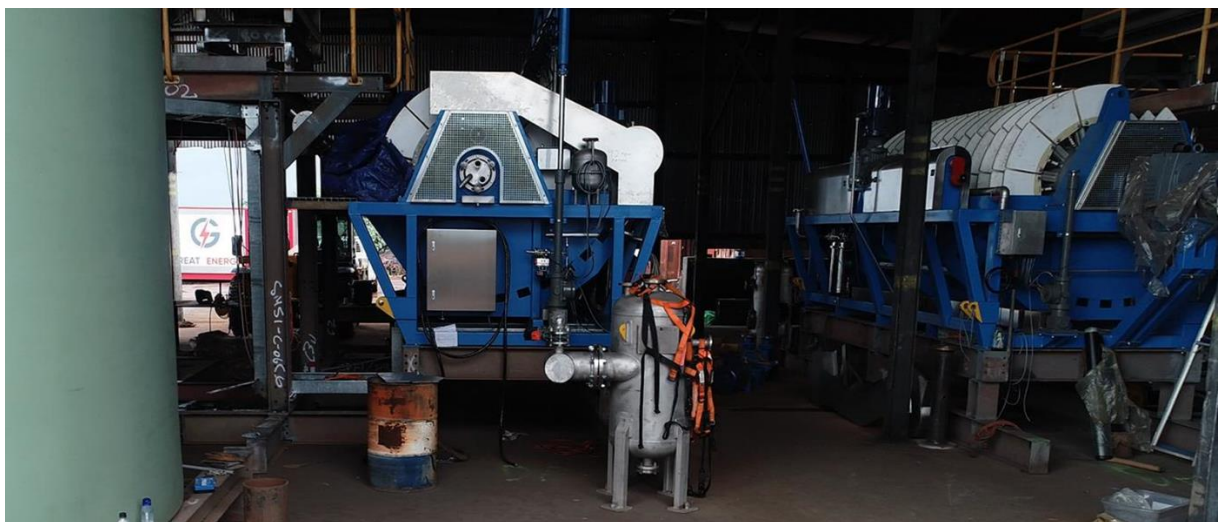
2 Ceramic Disk Filters for de-watering final product
