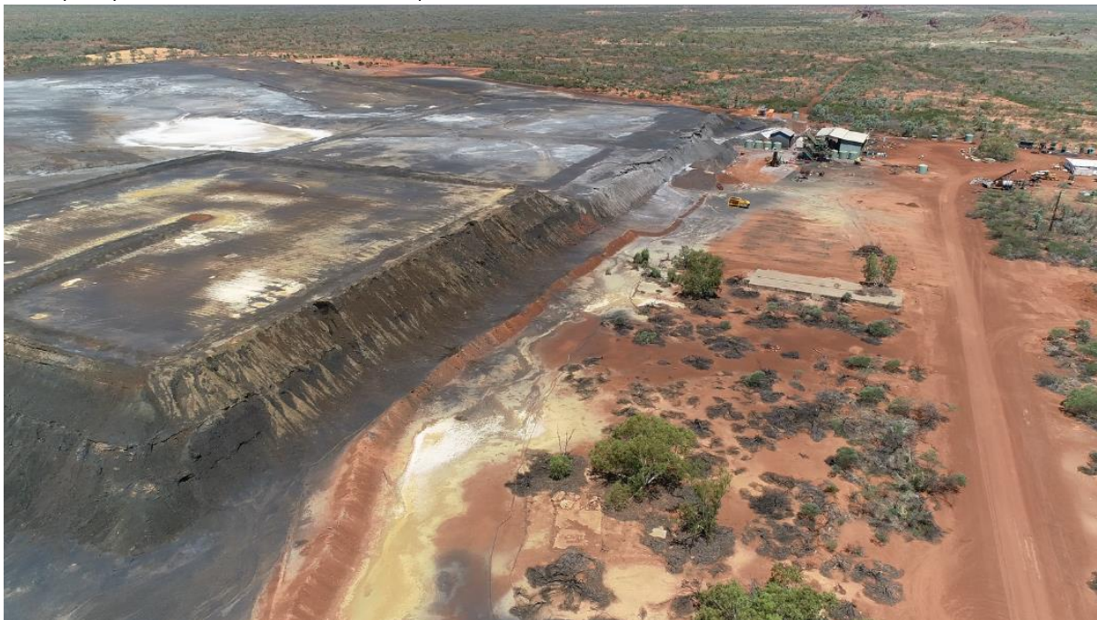
Peko Tailings and plant from the air. Tailings pile circa 500m x 500m x 9m high
