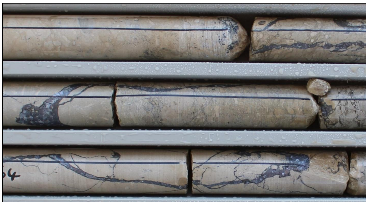
Figure 4: Sphalerite & galena-rich high angle-style mineralisation - EPDD2115: 1m @ 8.04% Zn + Pb from 38m.
