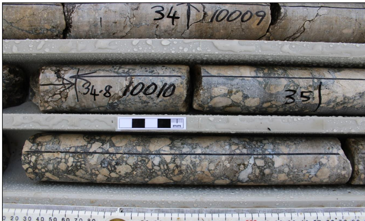
Figure 3: Sphalerite-rich breccia-style mineralisation - EPDD2101: 1.20m @ 4.28% Zn + Pb from 34.8m.
