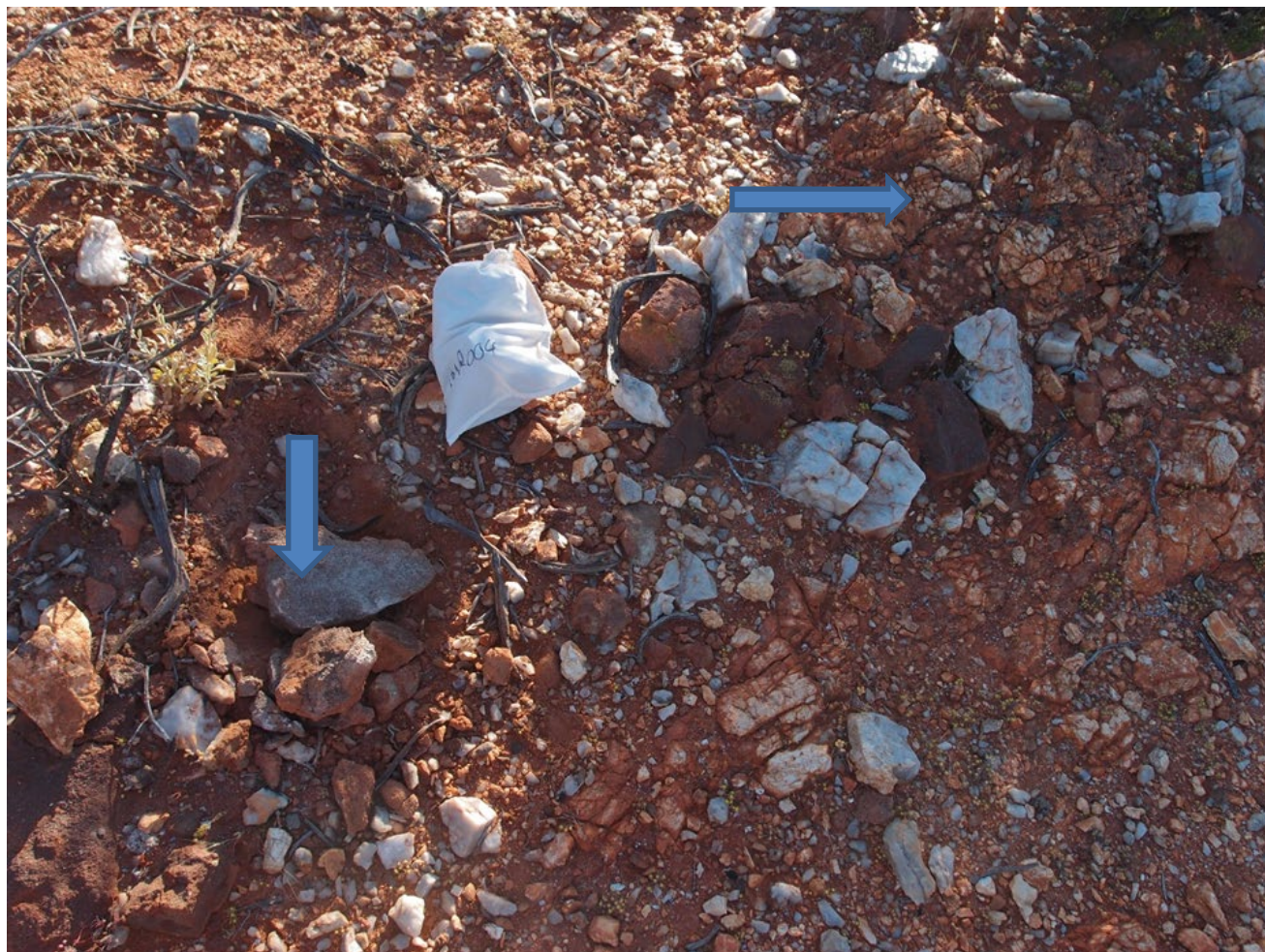
Figure 8. Rock sample NR0004, greisen-like morphology consisting of micaceous laths and microcline. Laboratory analysis reported 9,307ppm Rb and 0.32%Li and 1,934ppm Cs. Arrows indicate the sample outcrop and rock texture on a fresh face.
