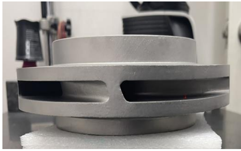
3MF Impeller printing in Hastelloy
