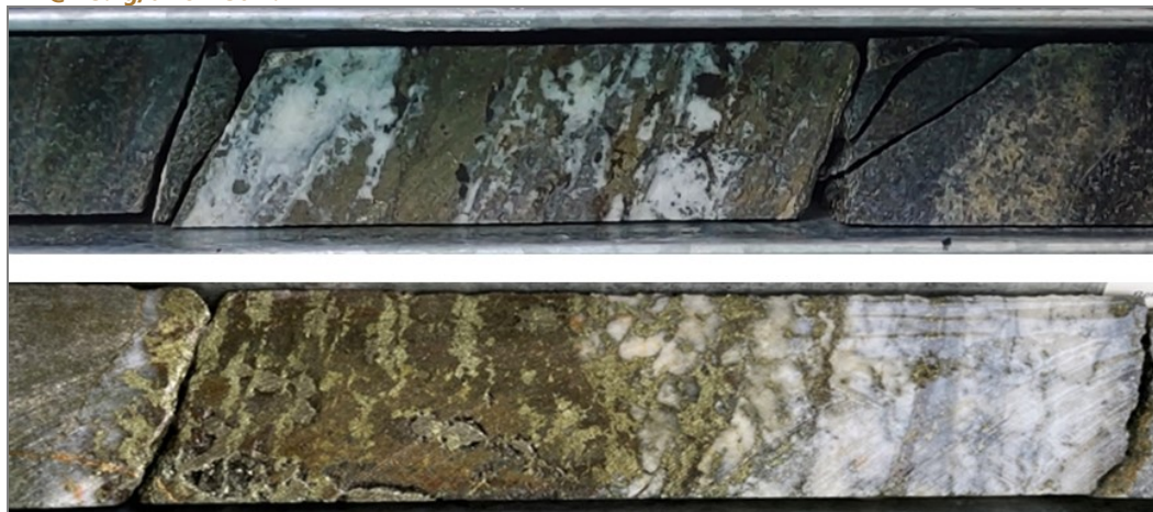
Figure 1 | Mineralised veins in Memot Diamond Core. Quartz veining with Pyrite, Arsenopyrite, Pyrrhotite, Chalcopyrite and Sphalerite sulphides. Top: DD21MMT0011m @ 7.76g/t from 51m, Bottom: DD21MMT005 1m @ 25.4g/t from 30m.
