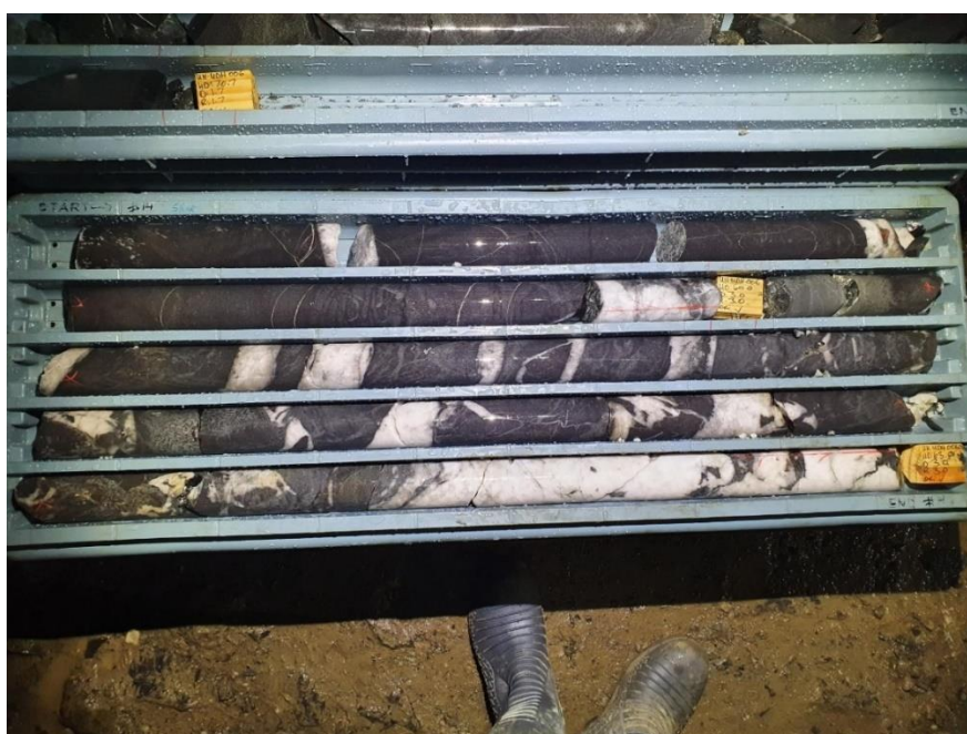
Image 2: Eaglehawk reef showing typical mineralised quartz/sulphide lodes, UH-UDH-006: 59.73m to 61.5m for 1.77m @ 29.6 g/t gold
