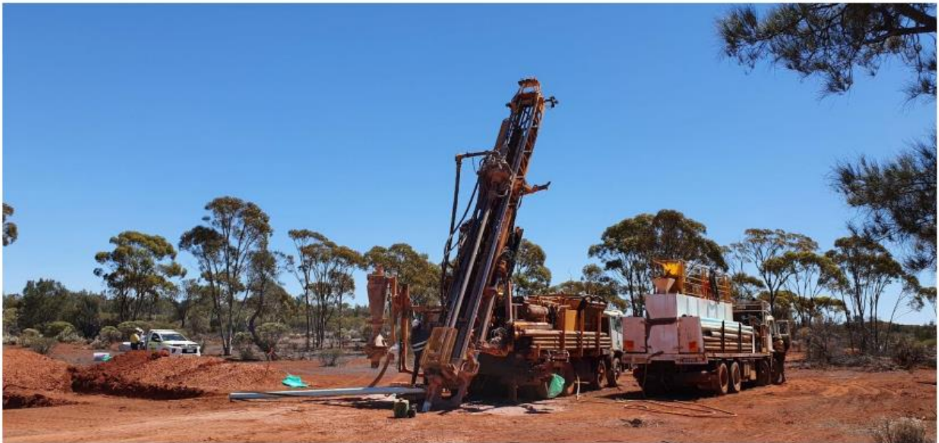
Figure 3: RC rig set up for drilling at Omrah nickel prospect
