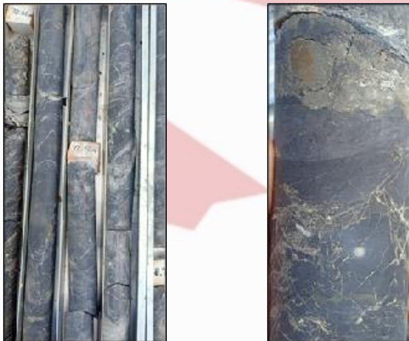
Figure 5 - Drill core showing typical sulphide related mineralisation within veining at JUDDH89 core (left) and close-up of a more intense zone of sulphide mineralisation in JUDDH90 (right)
