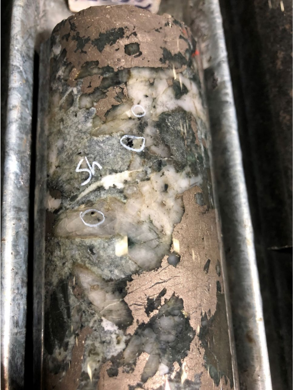
Figure 3 | Photo of mineralised skarn at 119.9 m in ML339M (Sh = Scheelite)
