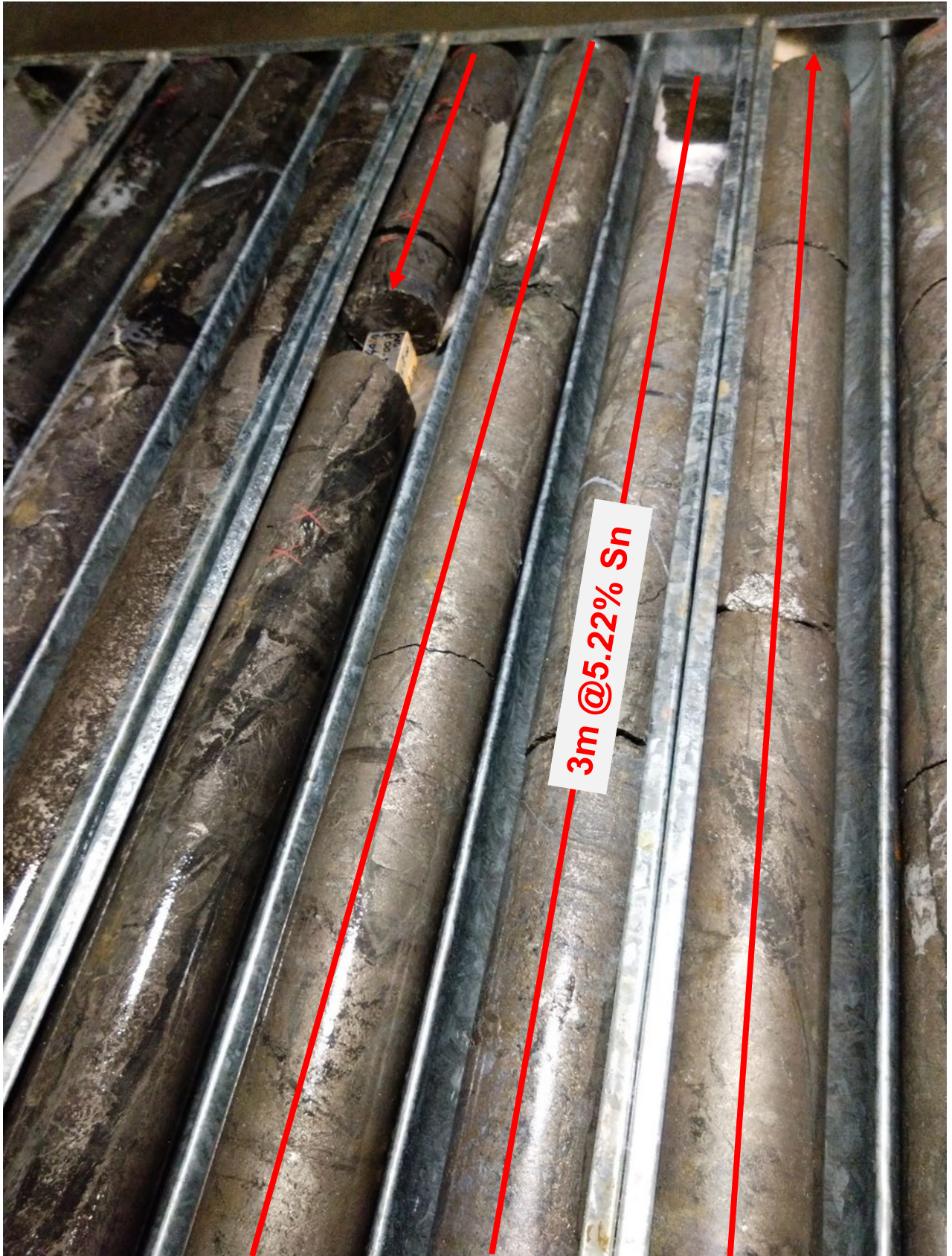
Figure 4 | Photo of mineralised sulfide rich skarn with 183-186 m assaying 5.2% Tin in ML340M
