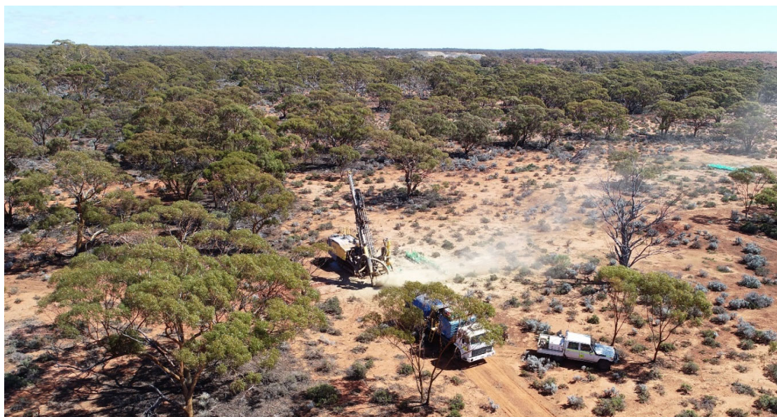
Figure 1: RC rig drilling extensional holes at Jones Find
