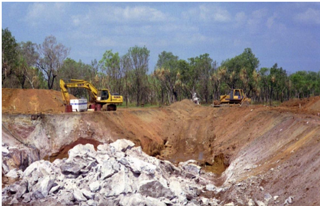
Figure 3 Test mining of magnesium at Winchester during the wet season (after blasting Level 0)
