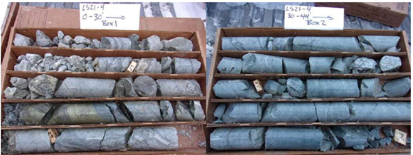
Figure 3: Drill hole LS21-004 from 0m - 13.41m (44ft), highlighting Upper Zone mineralisation intersected. Core blocks represent downhole depth in feet. Note: significant loss from 0-25ft due to drilling through unconsolidated overburden.
