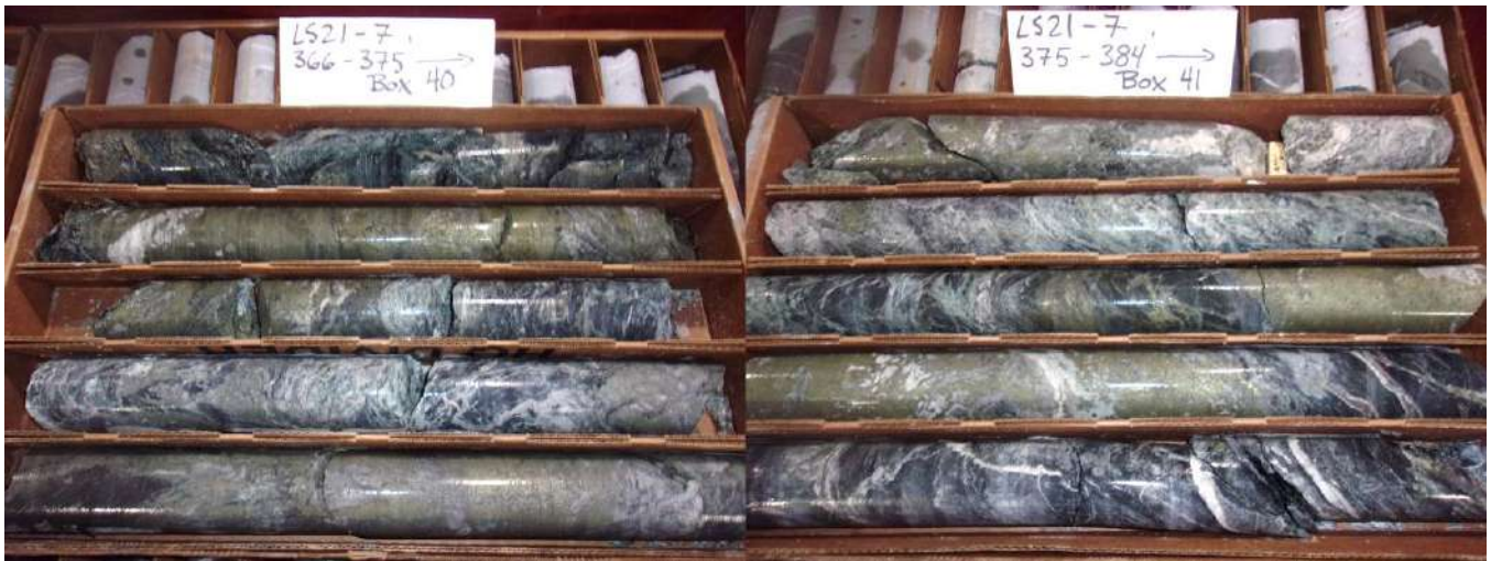
Figure 5: Drill hole LS21-007 from 111.57m (366ft) – 117.04m (384ft), highlighting Lower Zone mineralisation intersected. Core blocks represent downhole depth in feet.
