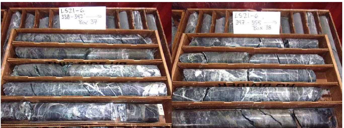
Figure 4: Drill hole LS21-006 from 103.02m (338ft) – 108.2m (355ft), highlighting Lower Zone mineralisation intersected. Core blocks represent downhole depth in feet.
