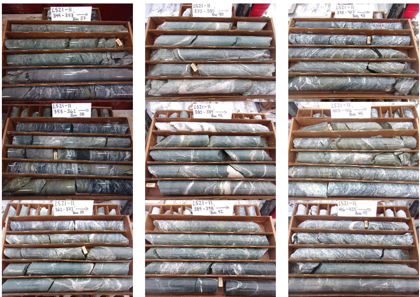
Figure 2: Drill hole LS21-011 from 104.85m (344ft) - 129.54m (425ft) highlighting zones of sulphides intersected on the eastern edge of the drilling program. Core blocks represent downhole depth in feet.
