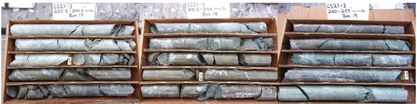
Figure 1: Drill hole LS21-003 from 70.87m (232.5ft) – 78.94m (259ft), highlighting observed quartz veins with massive sulphides. Core blocks represent downhole depth in feet.
