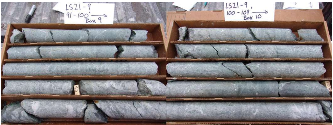
Figure 7: Drill hole LS21-009 from 27.74m (91ft) – 33.22m (109ft), highlighting rhyolite hosted, disseminated, Upper Zone mineralisation. Core blocks represent downhole depth in feet.
