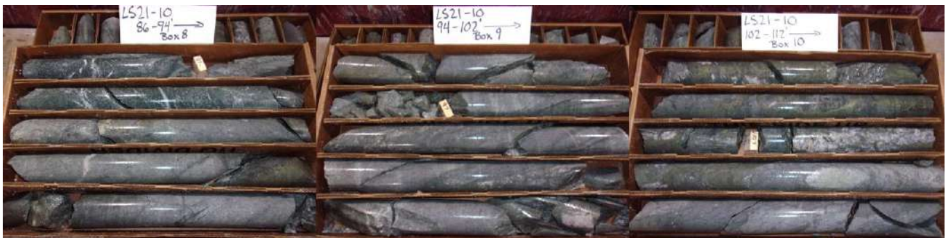
Figure 8: Drill hole LS21-010 from 26.21m (86ft) – 34.14m (112ft), highlighting rhyolite hosted, disseminated to locally massive, Upper Zone mineralisation. Core blocks represent downhole depth in feet.
