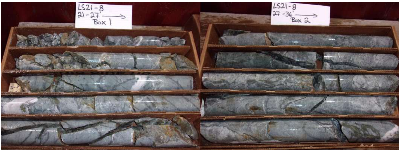
Figure 6: Drill hole LS21-008 from 6.4m (21ft) – 10.97m (36ft), highlighting Lower Zone mineralisation intersected. Core blocks represent downhole depth in feet.
