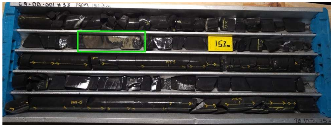
Figure 10 Coarse grained sulphides (highlighted in green) hosted in black shales. The photo shows hole depth 151.3m – 155.75m in CADD001.
