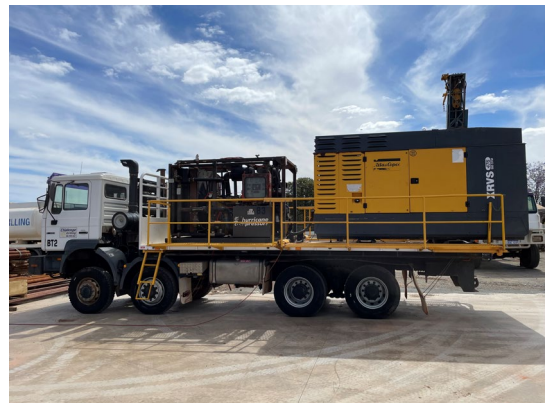
Image 3: Booster and Auxiliary Compressor Truck Delivered to Mt Chalmers Site.
