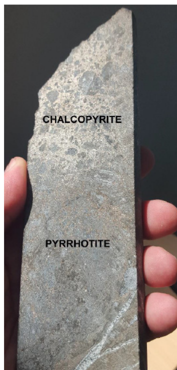
Figure 4 : Drill core pictured from T4GDD178 (124.65m) with chalcopyrite and pyrrhotite mineralisation intercept yet to be assayed
