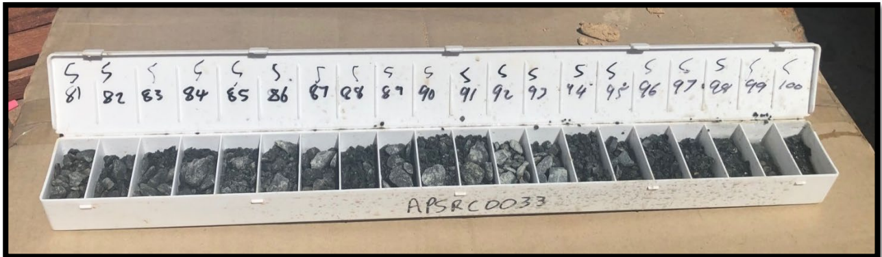
Photo 2: Chip tray from hole APSRC0033 depth 80-100m showing sulphides in a basaltic unit
