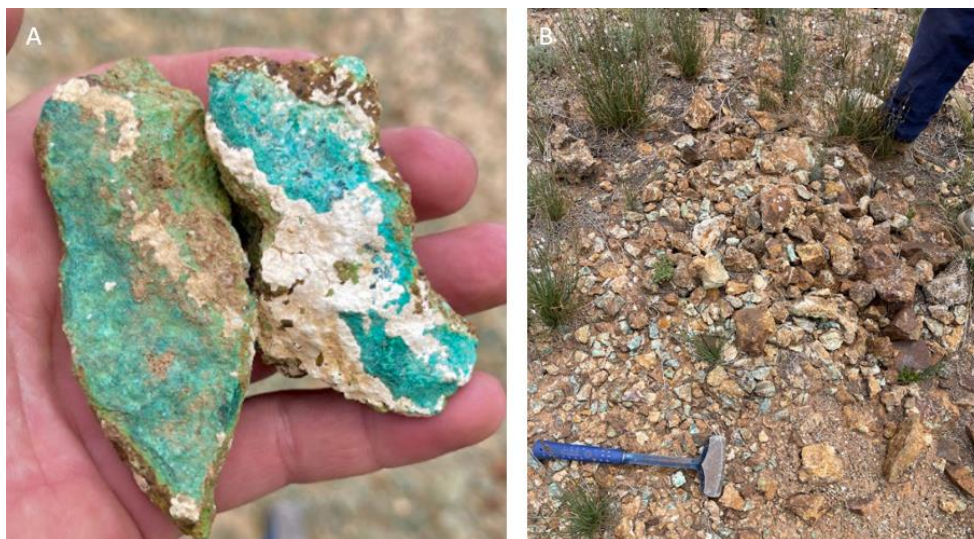
Figure 7. A) Sample 15550 which returned 41.1% Cu, 83g/t Ag, 0.17g/t Au; and B) Spoils from the historical workings.
