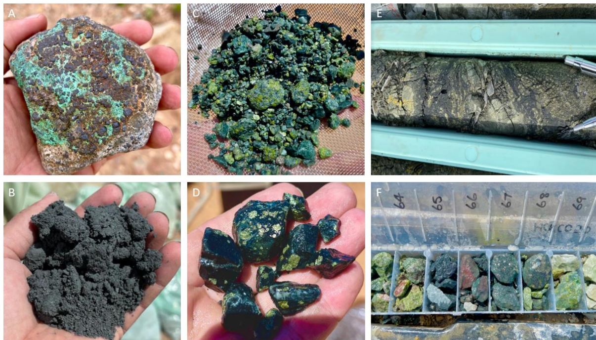
Figure 1. Hydrothermal Hill skarn system with (A) Copper enriched magnetite-skarn float (sample # 15730) B) Rich magnetite endoskarn from within MCRC049 at Hydrothermal Hill (120m depth, assays pending); C) Intense epidote alteration within mafic-ultramafic endoskarn (MCRC049, depth 60m, assays pending); D) Coarse disseminated chalcopyrite in exoskarn zone at Hydrothermal Hill (MCRC049 168m, assays pending); E) Magnetite endoskarn in MCDD004 45m depth; and F) magnetite-pyrite endoskarn from MCRC050 (64-68m, assays pending).
