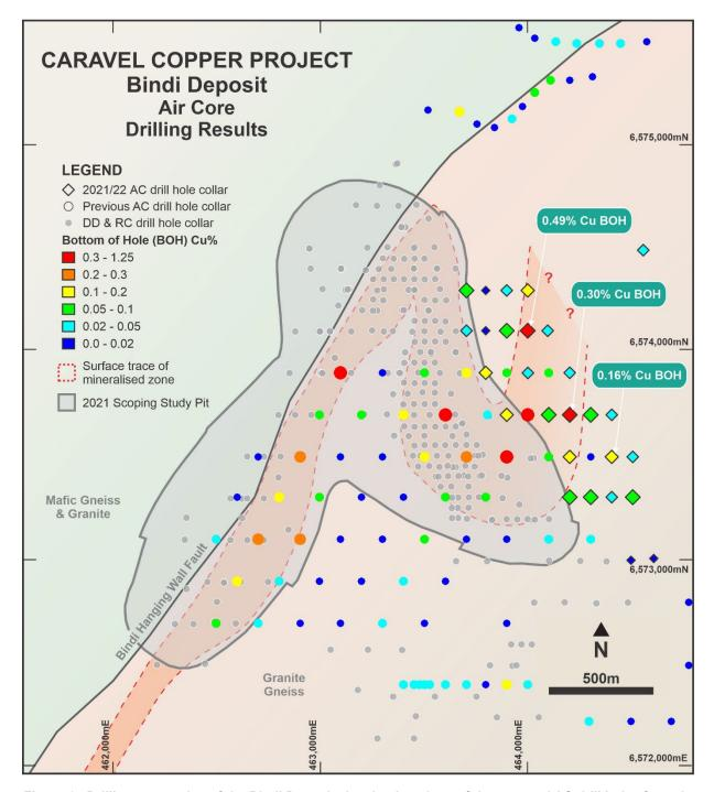
Figure 1: Drilling status plan of the Bindi Deposit showing locations of the reported AC drill holes from the 2021/22 program, previous AC drillholes, previous drill collar locations and the 2019 scoping study pit. All AC drill collars are coloured for the bottom of hole copper grade.
