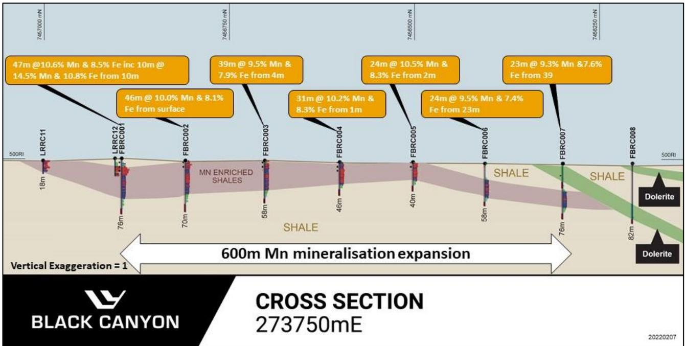
Figure 2. LR1 deposit cross section 273,750mE showing significant (looking east)
