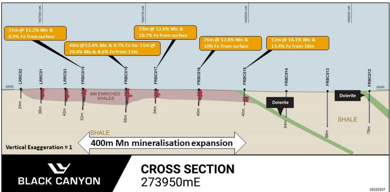
Figure 3. LR1 deposit cross section 273,950mE (looking east)
