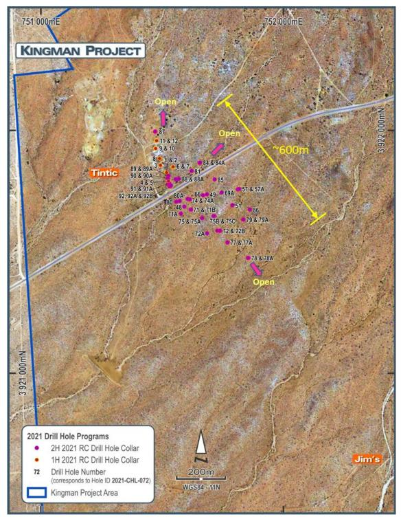
Figure 1 – collar locations of RC drill programs over the historic Tintic mine area and the extensional drilling to the south of the historic mine area. Arrows indicate direction of potential open mineralisation.
