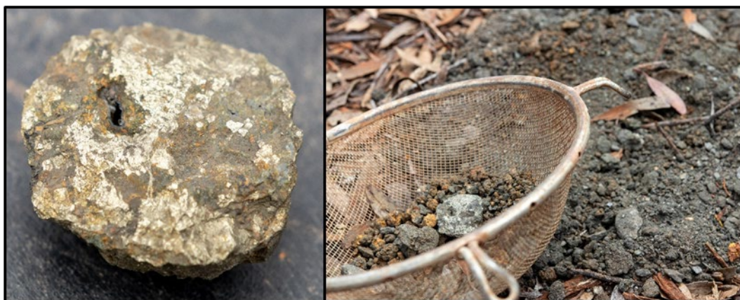
Figure 2 – Massive sulphide chip (25mm across) from 60m in NAC105. Bottom of hole sample pile on right.
